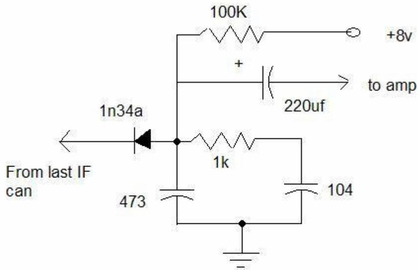
Audio was supposed to come off the top of the .1 cap, but I liked the level at the anode of the diode better. to take the audio from the oterh end of the 1oK resistor, reduce the size of the .1 capacitor to maybe .003 uf.
