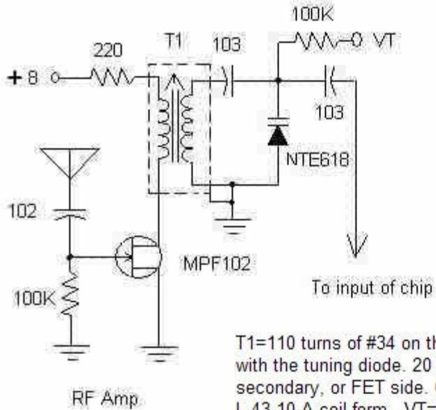
T1=110 turns of #34 on the secondary side, the side with the tuning diode. 20 turns #34 above the secondary, or FET side. On a CWS byemark L-43-10-A coil form. VT=9 volts for testing, and 8 volts from the RVG.
