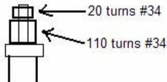
**10/06/06** I like this detector for the LM3820 better than the FET detector I had in the schematic.
