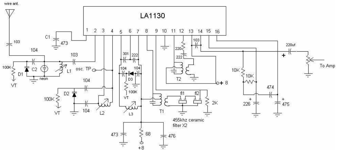
L1=75 turns on green (10.7 mhz) IF core-cut three pins off the one side.
