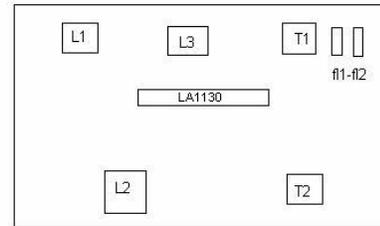
Keep oscillator coil away from RF sections.
